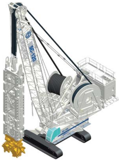
a) SOILMEC 'Tiger' series hydromill (hose drum design)
