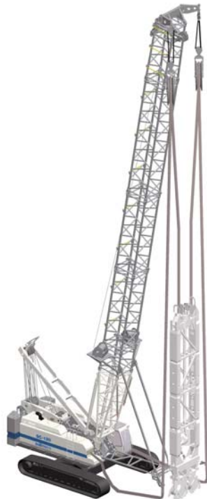
b) SOILMEC 'Cougar' series hydromill (hose wheel design)
